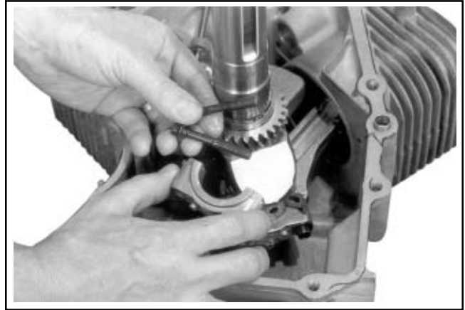
Figure 9-66. Mark End Cap with Cylinder Number Before Removal.
